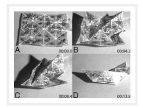
An experimental 'boat' self-folds as actuators receive current and magnetic closures engage.
