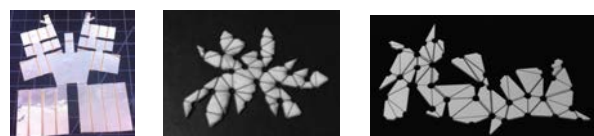
Fig. 11. Self-folding sheets (before bake) for humanoid (left), egg (center) and bunny (right)
